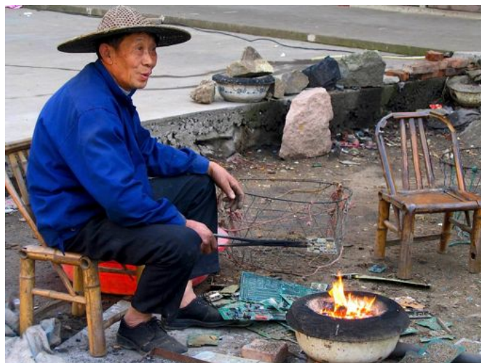
Fig. 3.1 Roasting of printed wiring boards over an open fire in Guiyu, China. Credit: Step Initiative / EMPA Source: http://ewasteguide.info/images/4333
